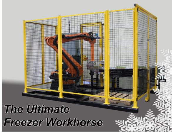
The freezer rated Polar Pal robotic palletizing system is a versatile and reliable unit. It can pick up and palletize case, bags, trays and just about whatever you need inside a -30 degree freezer room. It does not require any robot jacket or external heaters for it to operate in these conditions. Keep your employees out of the cold and let this system be the workhorse in your operation.
